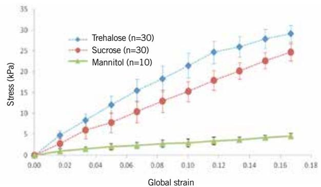
Figure 2: Mean maximum stress-strain curves for excipients processed using identical conditions; freeze-drying runs were carried out in triplicate for trehalose and sucrose (n=10 per run), single run for mannitol
