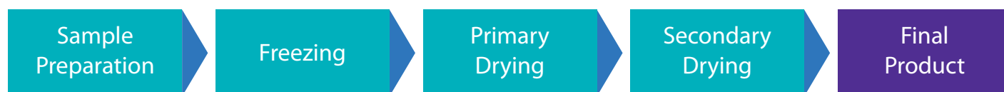
Figure 1: An overview of the lyophilization process
