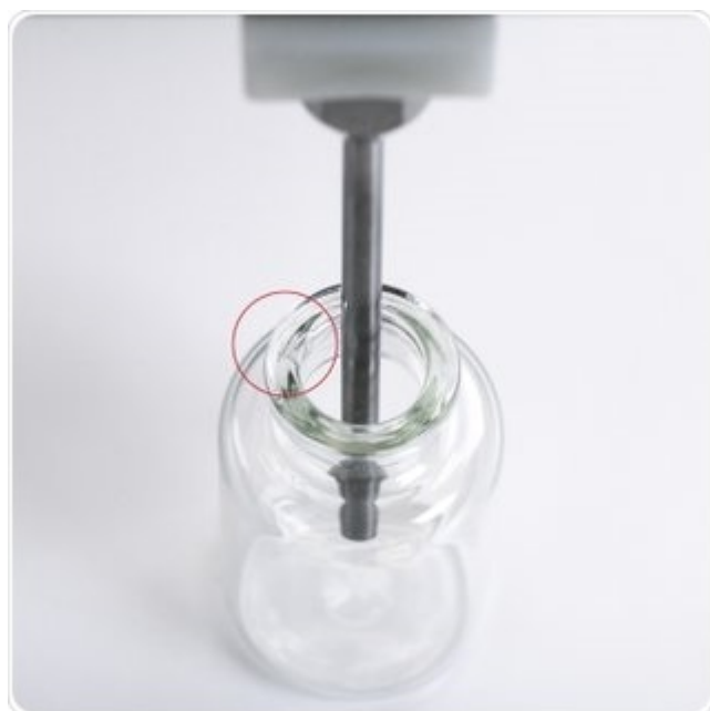
Figure 1: Chipped vial rim and resultant particulate generation. Image credit: SP Scientific
