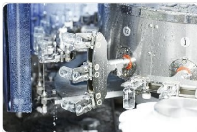
Figure 2: Modern washing and depyrogenation installation featuring washing needles. Image credit: SP Scientific
