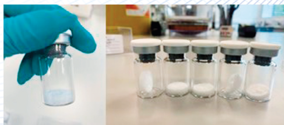
Figure 2 Controlled Nucleation at -8°C with a hold time of 20 minutes. Large bubbles were observed on the cake surface, indicating poor cake structure. The appearance did not meet the acceptance criteria.
