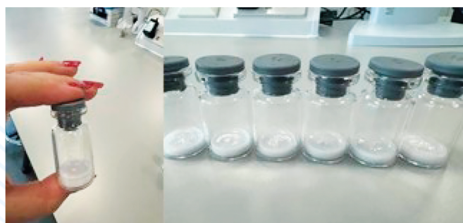
Figure 4 Controlled Nucleation at -20°C with a hold time of 20 minutes. White to off-white cake with no bubbles, smooth and glossy appearance, meeting the predefined acceptance criteria, suggesting that the applied process parameters led to improved cake structure and stability.
