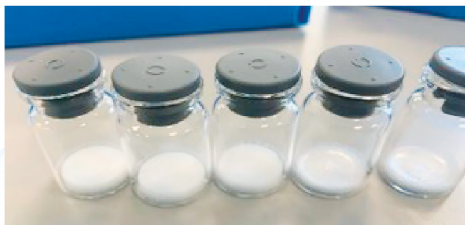
Figure 3 Controlled Nucleation at -15 °C with a hold time of 20 minutes. White to off-white cake with no bubbles meeting the predefined acceptance criteria, suggesting that the applied process parameters led to improved cake structure and stability
